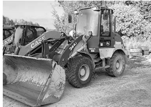
Deere 244J ldr., 12,000 hrs., eng. replaced @ 9000 hrs., $26,500.
